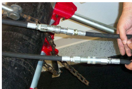
Lines attached to the hydraulic tool
